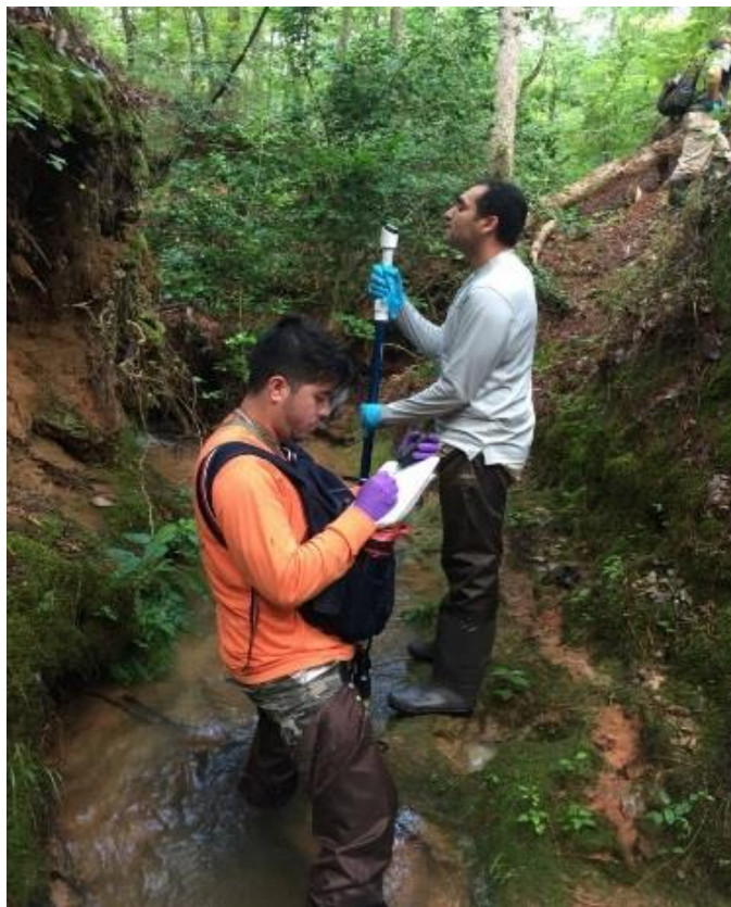
Figure 4: Measuring flow velocity using a flow meter.
