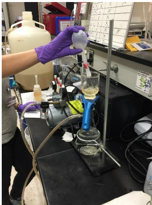
Figure 14: Preparation for laboratory testing at SREL: vacuum filtering of samples.
