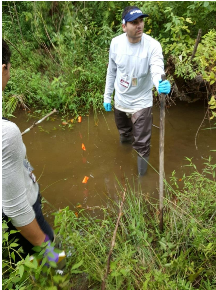
Figure 8: Flagging the segment across the stream cross section.
