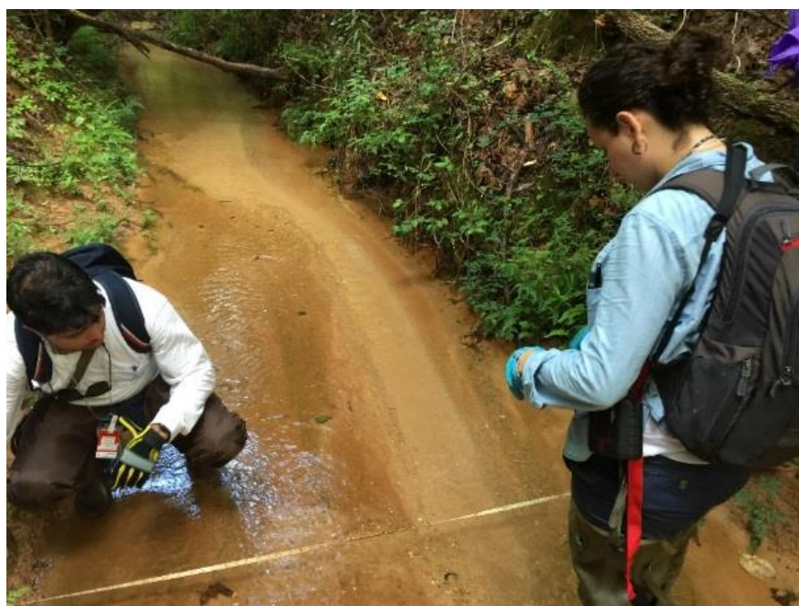
Figure 10: Manual measurement of stream width.
