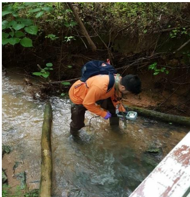
Figure 12: Water quality testing in Tims Branch using YSI multi-parameter meter.
